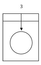
4. Keep pushing SLOWLY. Once the ball is **totally submerged** the upward force pushing back does not increase and remains constant, no matter how much deeper you push the ball into the water.
